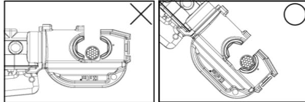
2. Pump the moving handle, the ram will rapidly advance. When the lower die makes contact with the terminal connector the tool will then slowly press the terminal until full compression is reached.
