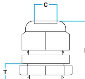
Supplied complete with a locknut and sealing washer to achieve IP68. For use with round cables.
